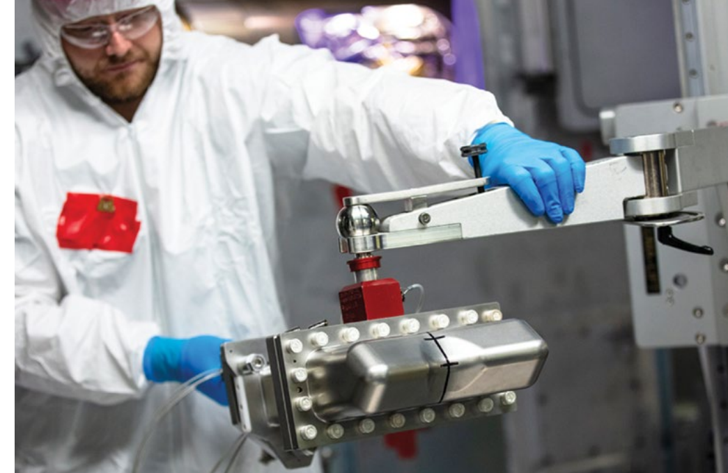
The cryogenic-compatible x-ray, neutron, and blast snout safely houses material samples to be subjected to fusion ignition irradiation environments inside a solid double-containment enclosure during a NIF experiment.
