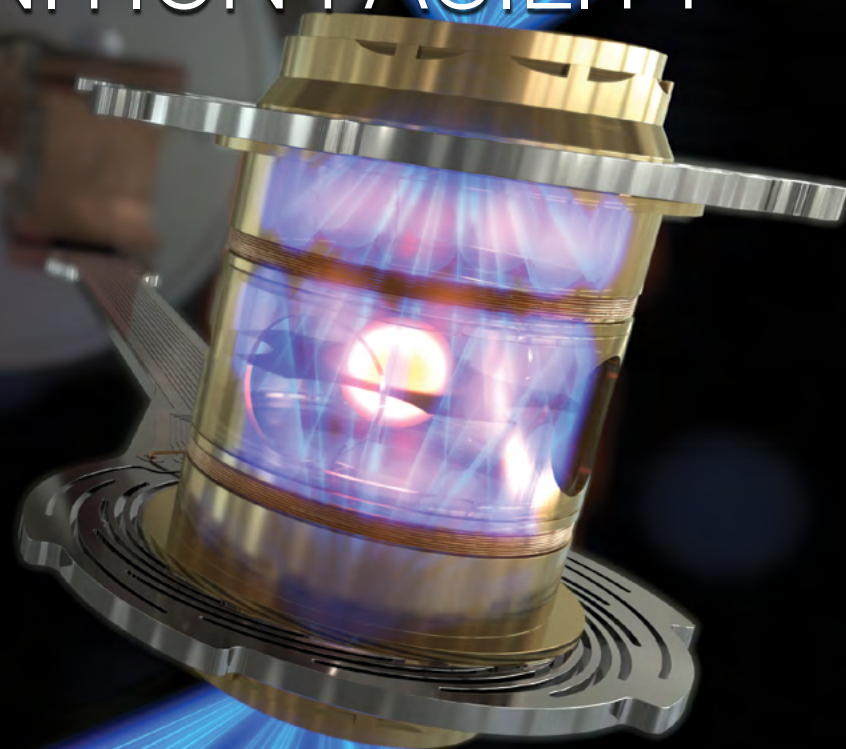
The decades-long quest to achieve fusion ignition and energy gain in a laboratory setting culminated with a NIF experiment that applied 2.05 MJ of laser energy to compress a capsule of deuterium-tritium fuel and produced 3.15 MJ of fusion energy.
