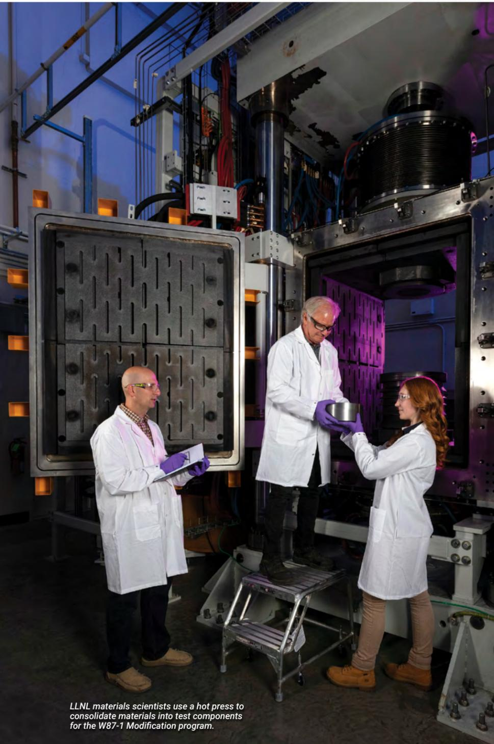
LLNL materials scientists use a hot press to consolidate materials into test components for the W87-1 Modification program.
