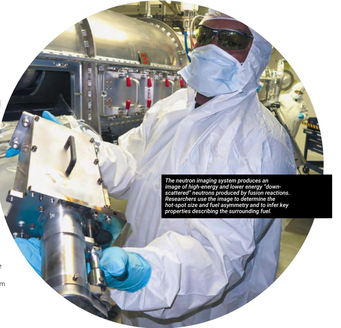
*The neutron imaging system produces an image of high-energy and lower energy "down-scattered" neutrons produced by fusion reactions. Researchers use the image to determine the hot-spot size and fuel asymmetry and to infer key properties describing the surrounding fuel.*
