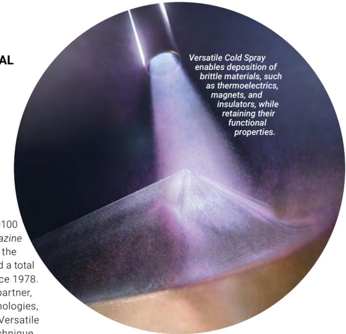
*Versatile Cold Spray enables deposition of brittle materials, such as thermoelectrics, magnets, and insulators, while retaining their functional properties.*
