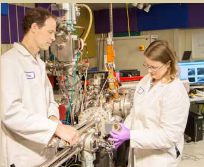
Livermore researchers Peter Weber and Jennifer Pett-Ridge prepare a sample for testing in the nanometer-scale secondary ion mass spectrometer (NanoSIMS), one of only a few such instruments in the world dedicated to isotope imaging in microbial biology and soils research.
