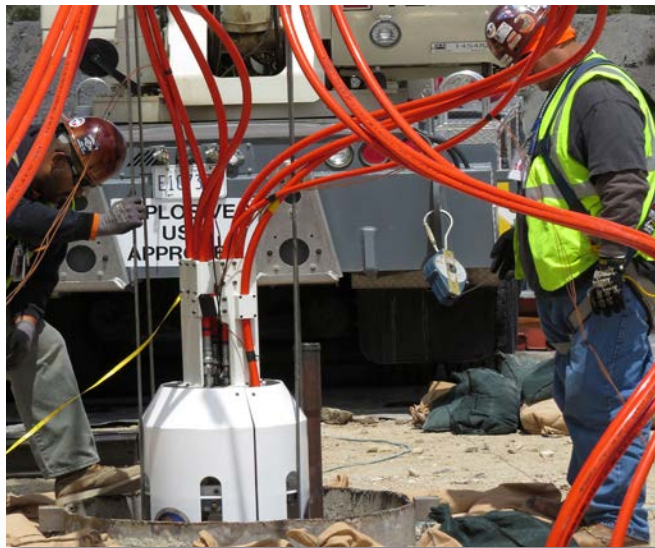
Two workers oversee the emplacement of the canister that contained the chemical explosive charge for Source Physics Experiment-4 Prime at the Nevada National Security Site. A chemical explosive equivalent to 196 pounds of TNT was detonated in the contained environment 286 feet below ground.
