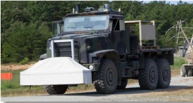
▲ A Laboratory team mounted its ground-penetrating radar system, iRADAR, onto an autonomous military cargo truck. The system received high marks in a field test of its ability to detect buried improvised explosive devices.
