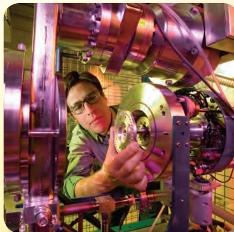
At Livermore's Center for Accelerator Mass Spectrometry, Ted Ognibene loads a sample in a tandem accelerator used mainly for biological research.
