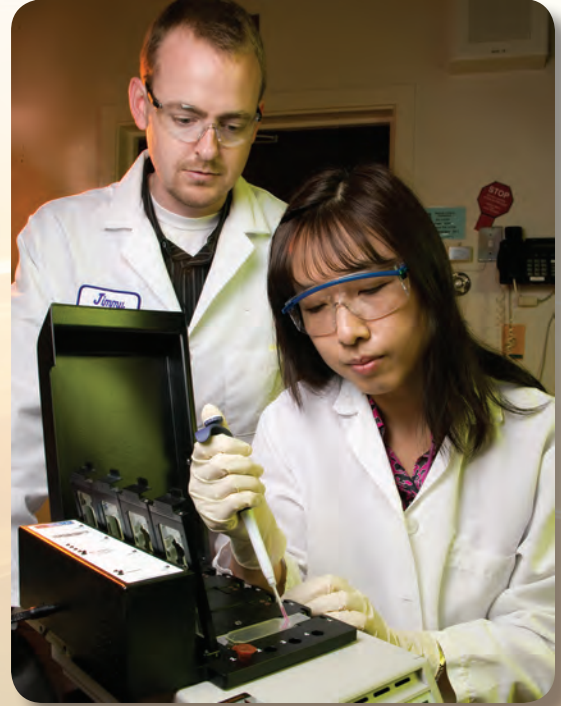
Biologists James Thissen (right) and Crystal Jaing work with a slide in the Lawrence Livermore Microbial Detection Array, which can detect greater than 5,000 different microbes.
